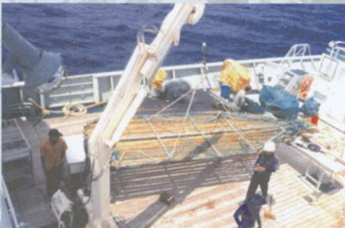
After covered by the sheet of fishing net to prevent the breaking of raft, the FAD is ready for launching
